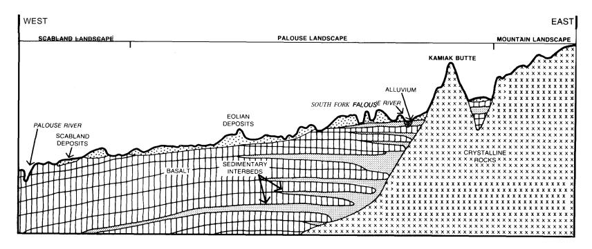
SCHEMATIC EAST-WEST GEOLOGIC SEC-TION THROUGH SOUTHERN WHITMAN COUNTY ADAPTED FROM WALTERS AND GLANCY, RECONNAISSANCE OF GEOLOGY AND OF GROUNDWATER OCCURRENCE IN WHITMAN COUNTY, WASHINGTON (1969), p.4.
