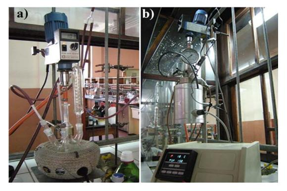
Lignin depolimerization was per-formed in a 0.5 L stainless steel reactor (Paar high pressure reactor; Paar Instrument Company, Moline, IL)
