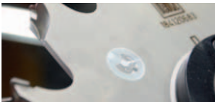
Tool with integrated data chip.
