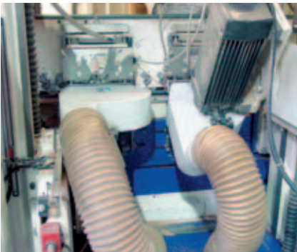
Problem: Machine wear through abrasive chips.
