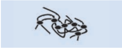
Structure of thermosets (schematic diagram)
