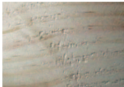
Finish planed surface after conventional preplaning.
