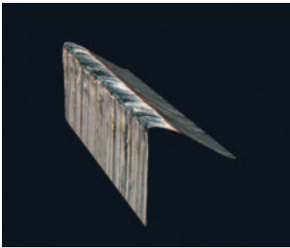
Sharp-edged wear on a coated HS edge.
