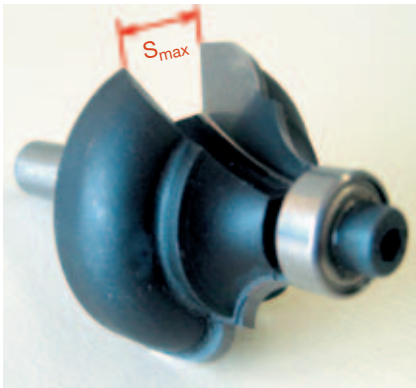
Cutting tool with guide ring for portable router.
