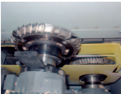
DFC® hogger with shredding edges shred the veneer projection on an extractable size for a complete disposal.
