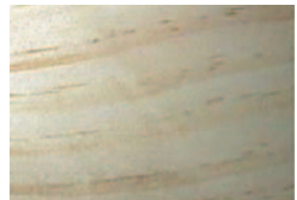
Finish planed surface after preplaning with RipTec.
