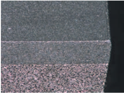
DP edge polycrystalline diamond layer (on top) sintered on to a tungsten carbide substrate (on bottom)
