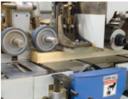
Detailed view of a four side planing and profiling machine with roller feed.
