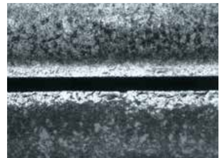
The cutting edges in the illustrations show the difference between abrasive wear (top) and wear caused by heat (bottom).
