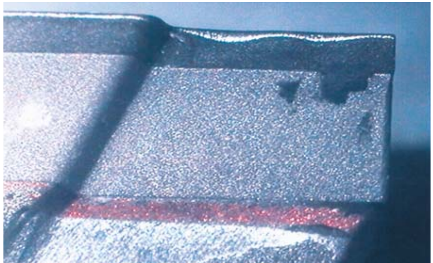
Cutting edge wear after machining GFK.
