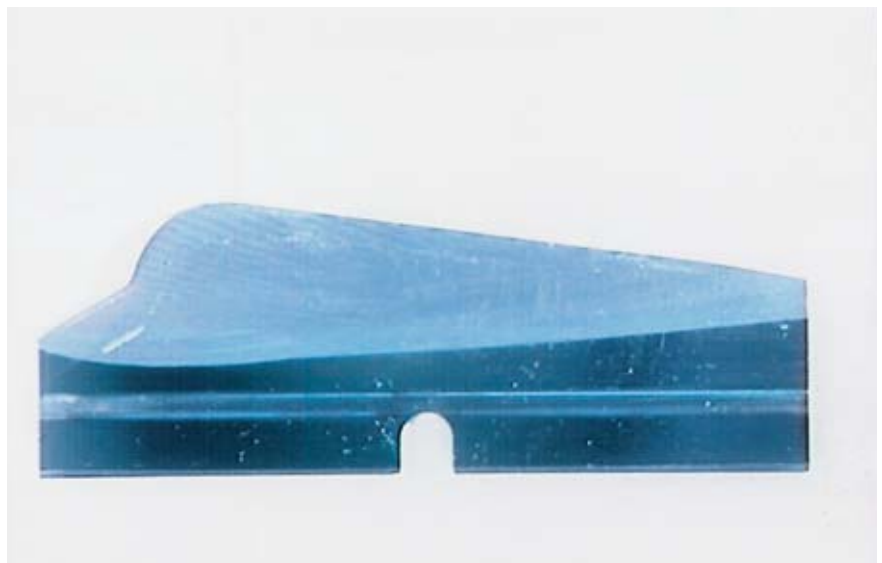
Damaged cutting edges due to incorrect repair.
