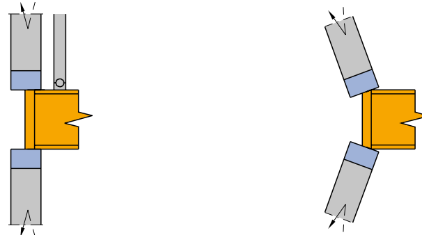
Trimming of edges on horizontal spindle - top motor tracing.
