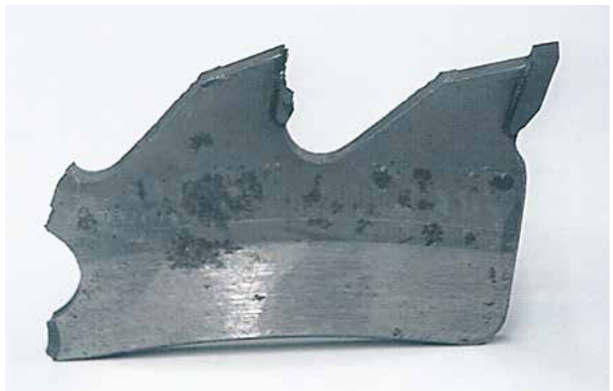
Destruction of saw tooth through overstress.
