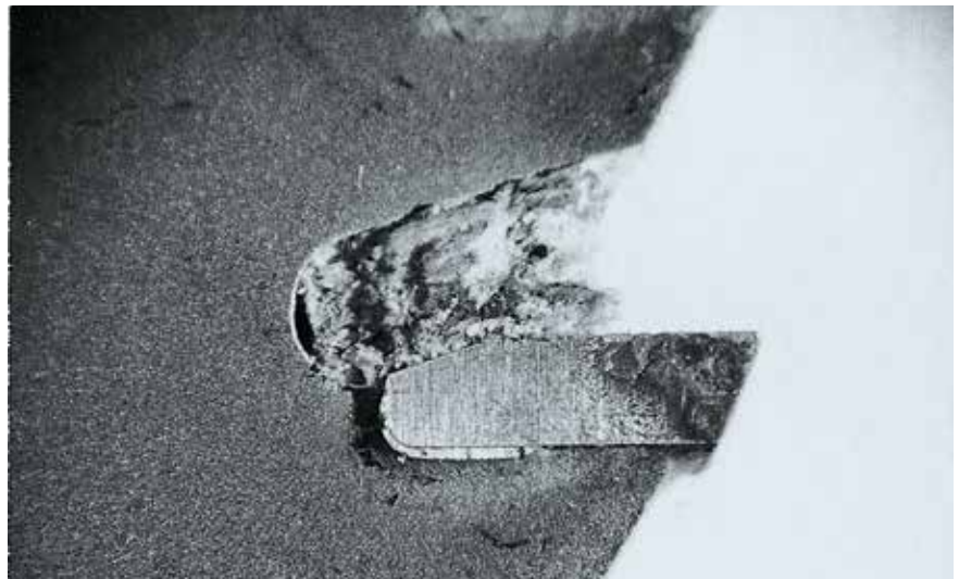
Cutting edge destruction through improper use.
